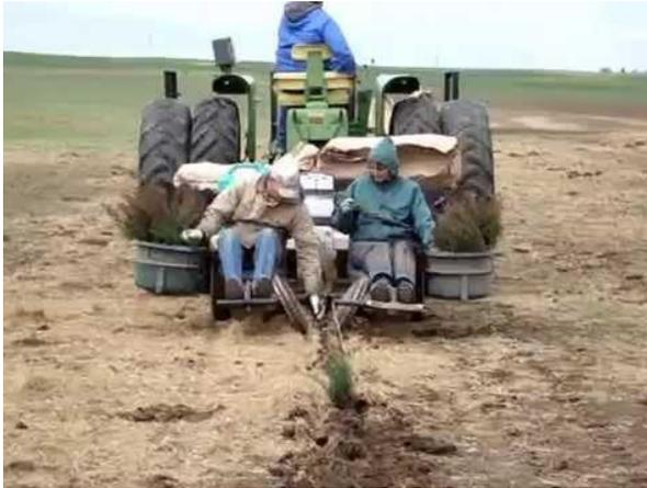
Figure 1: Knifing involves slicing the earth and a tree is deposited into the furrow, which is then packed by wheels.
