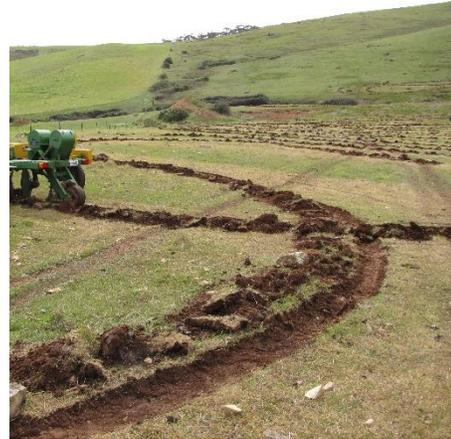
Figure 2: Scalping will leave a furrow with sod along the side similar to that shown above. The machine in use for tree planting, however, will also include a tree being planted with one pass of the machine.
